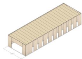
CLT box ~ 16m spans
